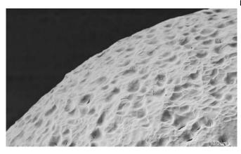
A stealth material surface, shown here, has been engineered to provide an "invisibility cloak" against the body's immune system cells. In this electron microscopy image, you can see the material's surface topography. Credit: Courtesy of the researchers
